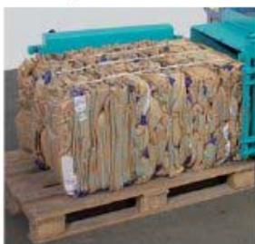
*KNL is a versatile horizontal baling press, available in 4 models. it easily compresses cardboard, paper, styrofoam, foils, tin cans, PET plastic bottles, plastic and aluminium containers, paint pails and metal barrels up to 60 litres (200 litres light barrels with KNL 160).*
