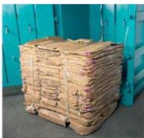
*the multi-chamber baler serves to sort and compress various material and offers maximum efficiency. the press ram is warp-free due to the AWS system, patented and designed by austropressen.*
